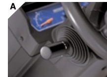
A Electric FNR Lever (Automatic Transmission Models)
