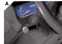
A Electric FNR Lever (Automatic Transmission Model)
