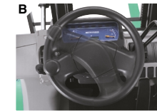
B Power Steering With 100% Standstill Steering
